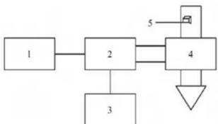
[Abstract] The characteristics of microwave drying equipment for three common commercially available wet rice noodles were studied. The results show that the water content of rice flour is related to microwave power and drying time. The higher the power, the longer the drying time and the lower the water content. The drying rate of rice flour is proportional to the microwave power. Drying with medium fire can be done in a short time. Get better quality rice noodles.
