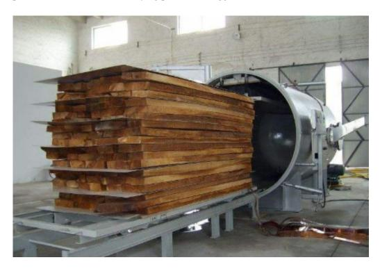
The working theory of wood microwave drying and insecticidal equipment:
